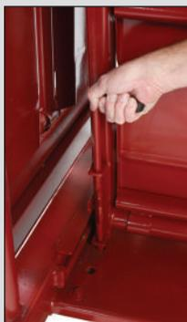
b. Top Width: Using squeeze release mechanism, release squeeze and pull up or down on large squeeze handle to get desired top width. It should be fairly wide when catching cattle and then squeeze applied after animal is caught.
